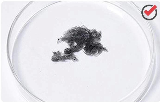
Cotton fiber burns out and turns into ashes
