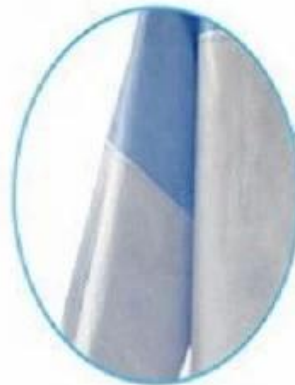
Ultra-sonic heat sealing seams
