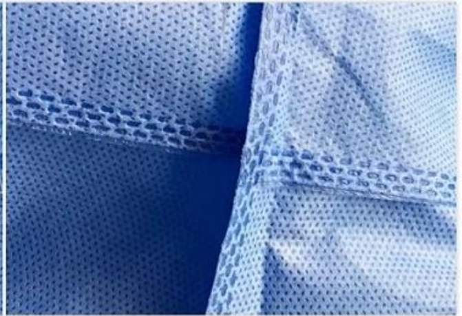
Ultrasonic sealing seams
