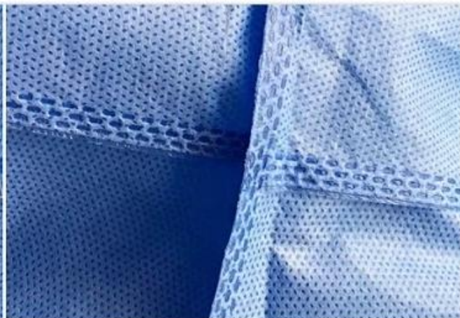
Ultrasonic sealing seams
