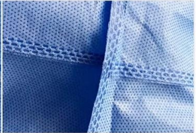
Ultrasonic sealing seams
