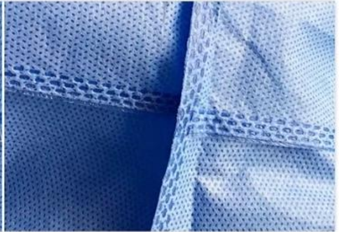
Ultrasonic sealing seams
