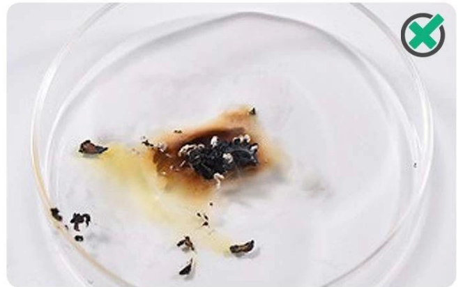
Chemical fiber will become black solid object after burning out
